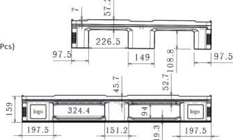
All dimensions may vary ±5 mm due to the production process & raw material characteristics.
